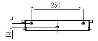
• Fix the mounting bracket as the figure shows. Do not make the screws to be flush to the wall. Instead, leave 2 to 4mm exposed.
