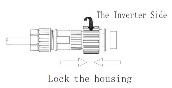
5:To remove the AC output terminal, press the bayonet out of the slot with a small screwdriver and pull it out, or unscrew the threaded sleeve, then pull it out.
