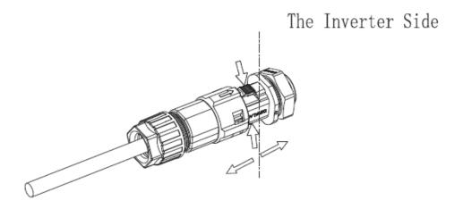
**Step 2** Insert the H type tool and pull it out from the socket.
