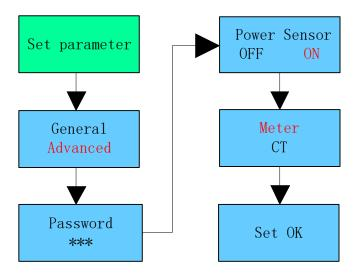
If you only want to check the load consumption function, you can choose Meter as Power sensor.CT is just only for Export Limit function.
