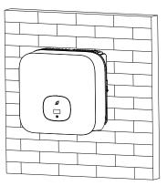
After confirming the inverter is fixed reliably, fasten one M6 safety-lock sockets head cap screws on the right or left side firmly to prevent the inverter from being lifted off the bracket.
