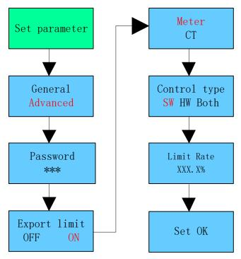
Under the permission given by your energy provider, the ratio of your system output power divide d by the rated power of the inverter is called Limit Rate.For instance,if the energy provider only accepts 4kVA/kW from your 5kW system, then the Limit Rate of 5kW inverter is 80.0%.
