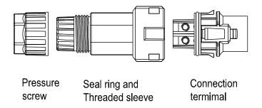
2. Insert the stripped and bared cable through pressure screw, seal ring, threaded sleeve in sequence, insert cables into connection terminal according to polarities indicates on it and tighten the screws firmly. Please try to pull out the wire to make sure the it's well connected.
